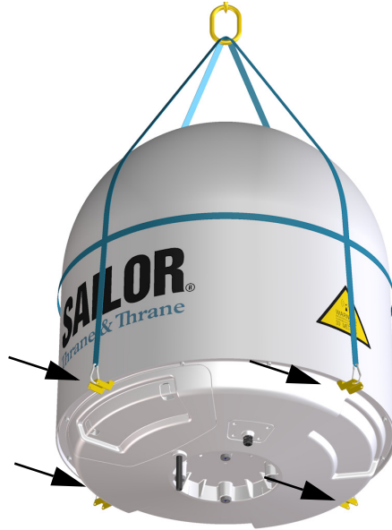
Figure 3-16: ADU installation, webbed sling attached to the 4 lifting brackets
