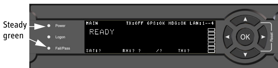
Figure 5-3: ACU display after first power on (example with LAN ports 1 and 4 used)
